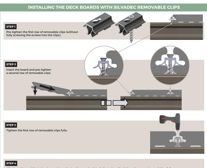
After inserting and fastening the next board using the standard single fastening clip, tighten the second row of clips fully. Repeat these operations for each row of boards which must be removable.
