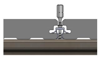
The removable clip is designed so that the screw is accessible with a standard Torx T15 bit.
